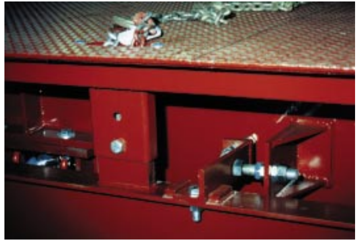
Conveniently located side and end bumper checking mechanism dampens motion in the deck and protects it from shock..
