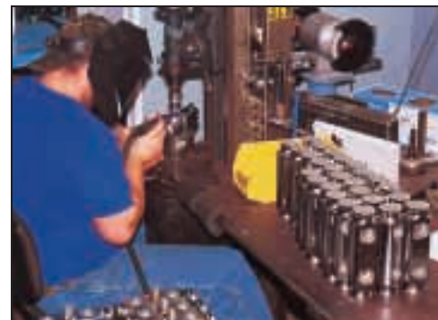
Specialized equipment and skilled technicians are used to TIG weld environmental seals on load cells.
