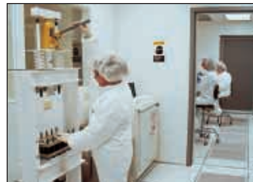
Strain gages are produced under strict clean room conditions.
