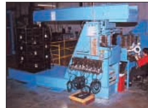
A number of dead weight testers are used to verify load cell performance
