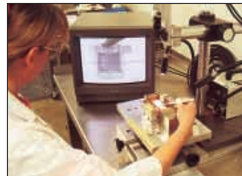
After bonding, strain gages and associated components are checked for proper alignment and adherence to the sensor body.
